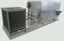
One of 52 custom units used for air conditioning a prison in Nevada. The design includes indirect-direct evaporative cooling for summer comfort and heat recovery supplemented with HW heat for winter heating.
