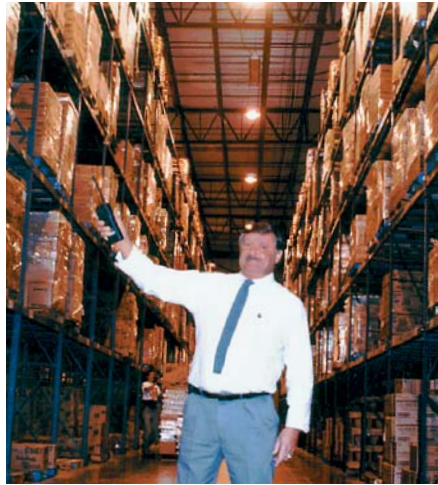
Left: Steve Cox points to a frost-free environment inside the Shaw's distribution center. Right: Before the installation of Munters DryCool equipment, frost build-up near exits formed blocks of snow and ice that threatened product quality, and forced workers to waste time chipping and thawing for hours every week.
